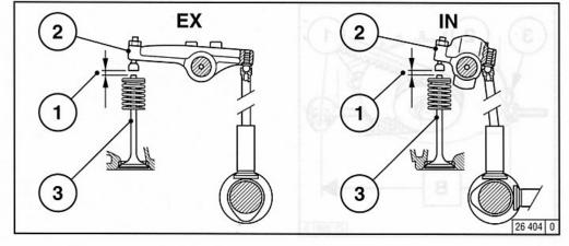
Check valve clearance 1 between rocker arm/ tappet contact face 2 and valve stem 3 with feeler gauge (there should only be a slight resistance when feeler blade is inserted).
